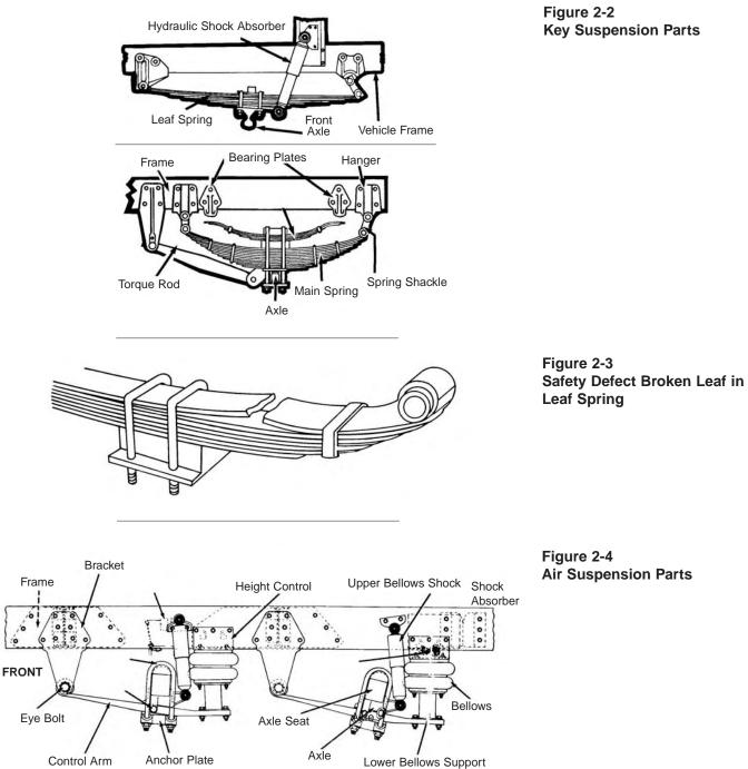
Figure 2-2 **Key Suspension Parts**
